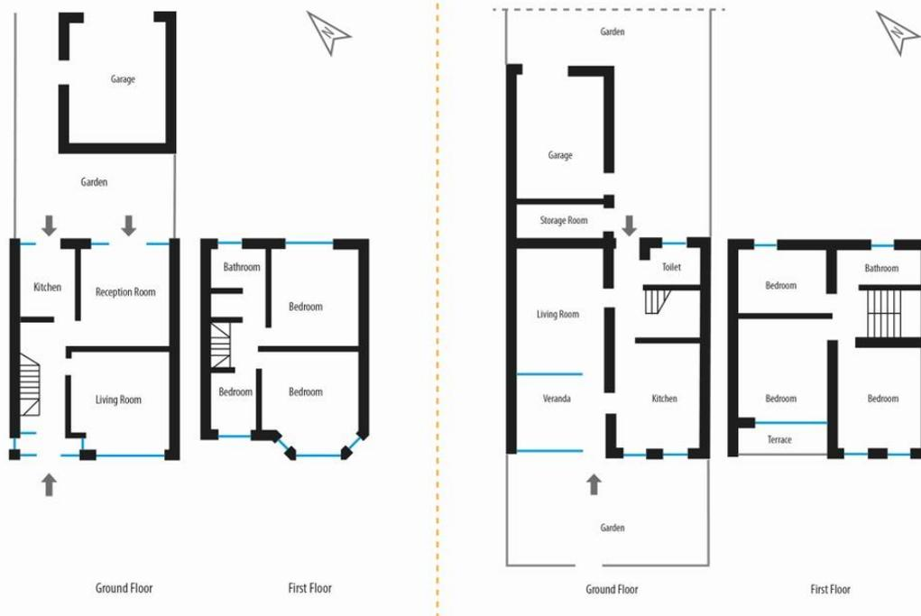
**Figure 3:** Houses plan- a) Wembley, College Road HA9; b) Pirot, Tigar factory housing (Drawings: Mirko Stanimirovic)
